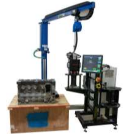
Bore Cylindricity Scanning Incometer
