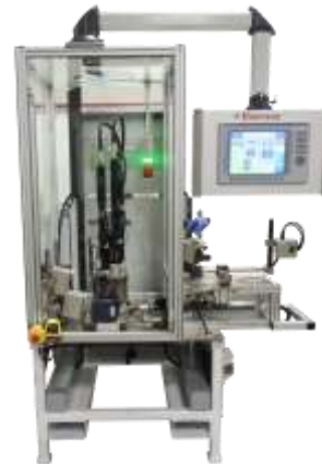
Semi-Automatic Torque & Tape Application System
