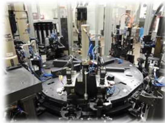
Multi Operational Indexing Systems for Multi Step Assembly
