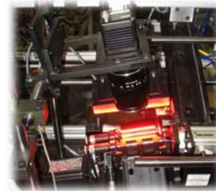
In-line Porosity & Surface Defect Inspection
