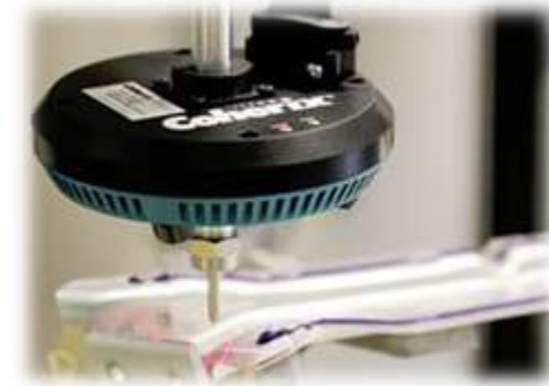
3D Measurement & Verification of FIPG Bead
