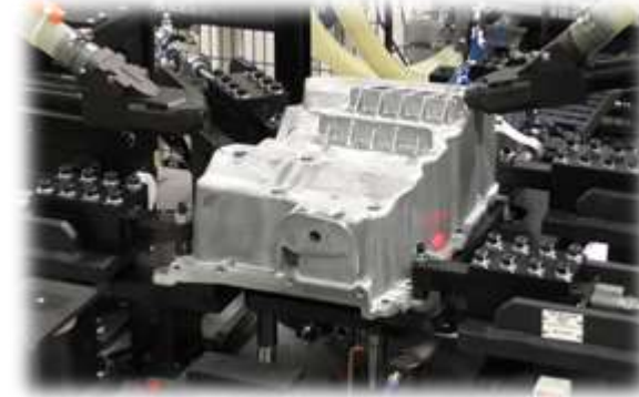
In-line Auto Torqueing & Dowel Pressing
