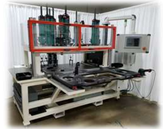
Semi Automatic Air / Oil Bushing & Dowel Press
