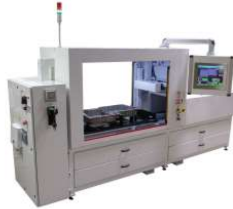
Battery Tray In-line Pre-Machined Straightening Non-Contact Gage
