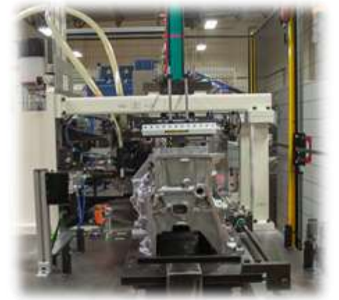
Semi Auto Glue Application & Cup Plug Installation
