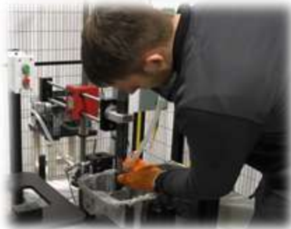
Manual Torque Benches with Blow Fed Subcomponents
