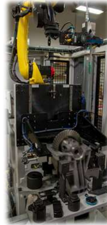
In-line Robotic FIPG Application & Inspection
