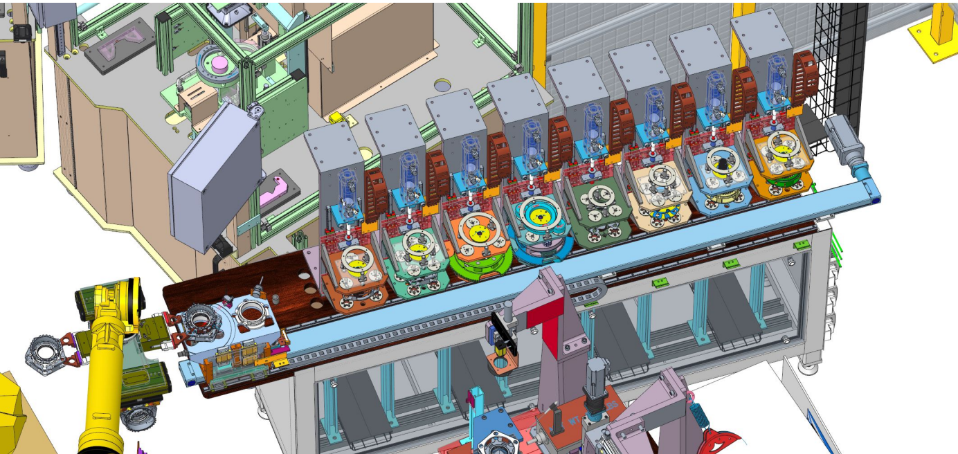
Multi Station Air Gage System with Servo Belt Drive
