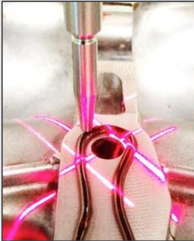
Powertrain RTV bead inspection
